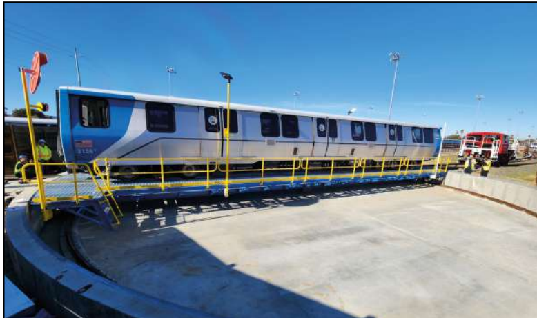
Bay Area Rapid Transit Authority Railcar Turntable
